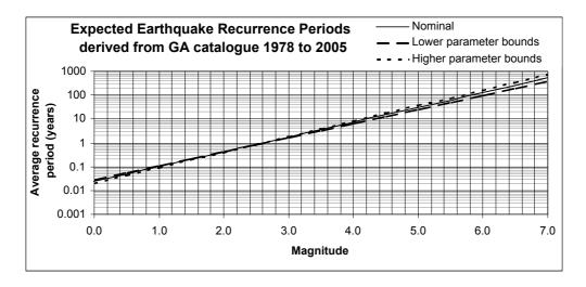
Figure 2: Expected Earthquake Recurrence Periods derived from GA catalogue 1878 to 2005
